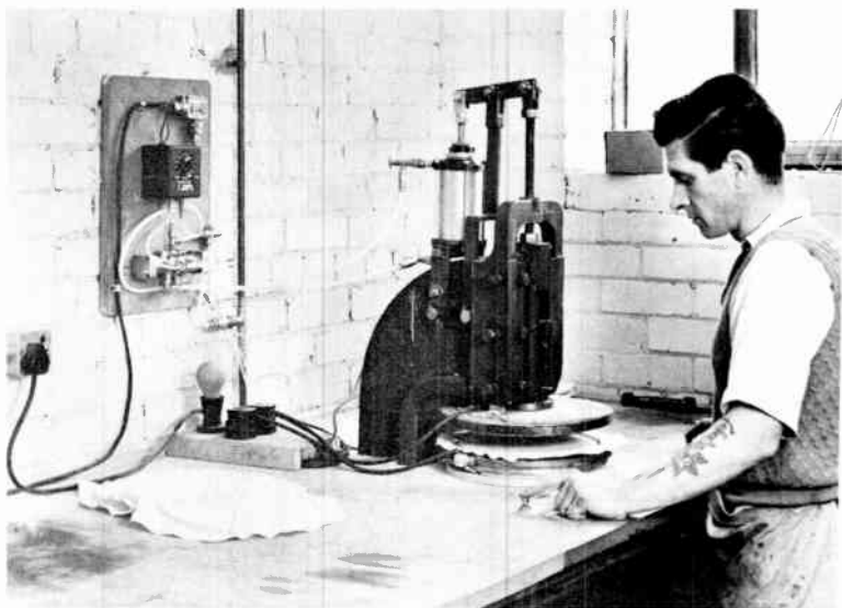
FIG. R/19B. Pneumatically operated and timed moulding press.
