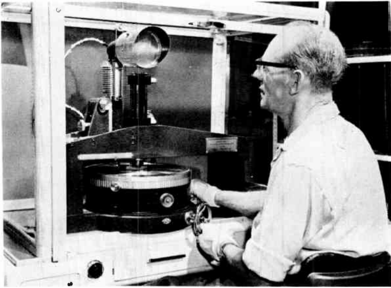
FIG. S/15. Machine for exact location of centre hole in metal master in relation to groove spiral.
