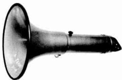
FIG. M/A. Modern megaphone complete with mic., transistor amplifier, volume control and re-entrant horn loud-speaker, capable of magnifying the human voice 100x.
