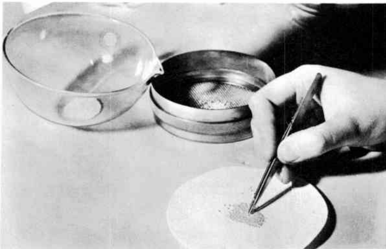
FIG. T/15. Sorting and inspecting the indium pellets for the emitters and collectors of transistors.
