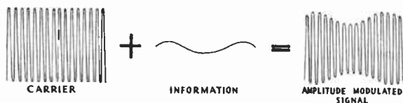
FIG. A/1. Amplitude modulation.
